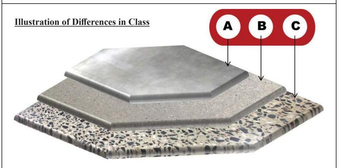
Caution: This provides a visual representation of the differences in Class A, B and C. This may not represent the polished concrete in your area as it varies based on aggregate type, gradation, size and distribution. Consult with your CPC Polishing Contractor to see reference samples or mockups.
